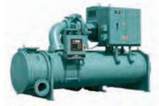
YK HP Water to water heat pump Centrifugal compr. / R134a Hot water up to 50°C (Std) Hot water up to 70°C (HP) Heating cap.: 1000 to 9000 kW
