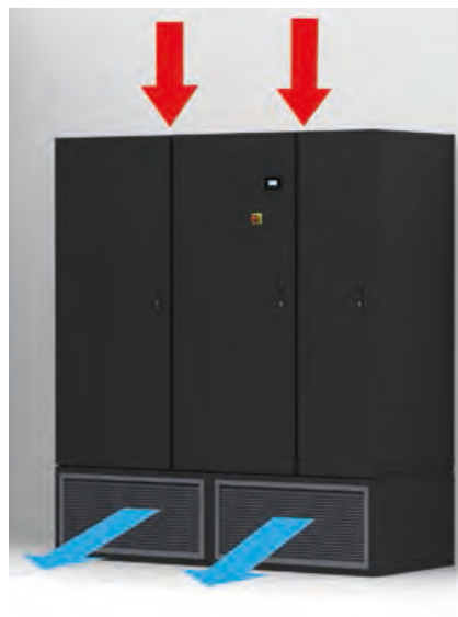
Suction with upper air intake and front air outlet with distribution plenum with adjustable grilles.
